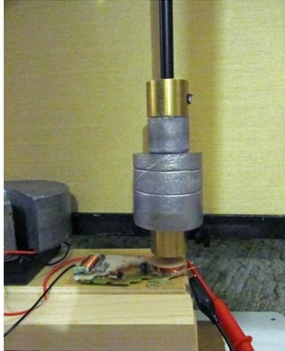
Furthermore, the flag's large dissipation renders the varying drag of the various bob masses negligible. As seen below, the pendulum was stopped after each attainment of equilibrium and free decay, and an additional mass added. Note the amplitude decreased with increasing mass!
