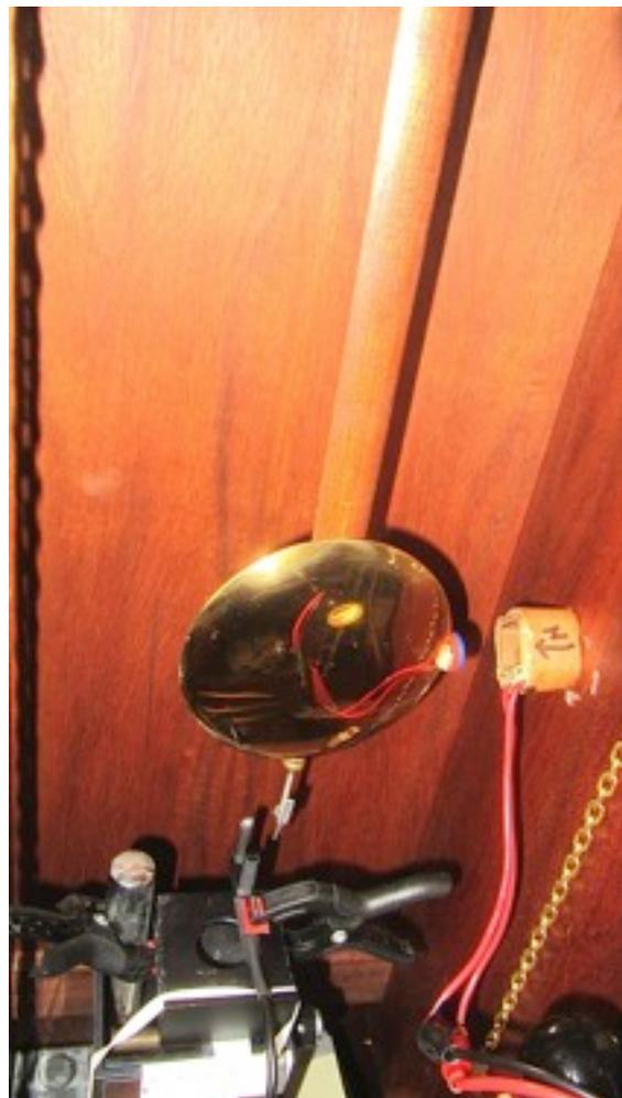
I found the bandwidth (FWHP) by finding the frequencies, using a quadratic fit, for double the EMF required to maintain the same amplitude as that at resonance. The following graphs are of the three trials:
